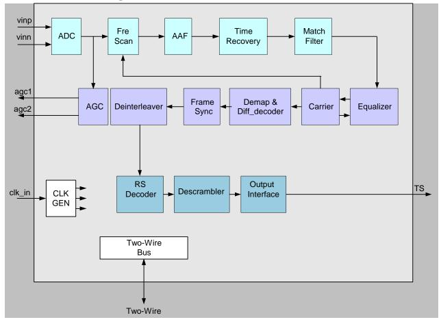
The Hi3130 is a single-chip cable digital TV channel receiving chip. It is compliant with DVB-C (ETS 300 429), ITU J83-A and ITU J83-C specifications. The Hi3130 provides powerful 16/32/64/128/256-QAM demodulation and forward error correction capabilities. It is intended for the complete processing toward cable digital signals, from IF sampling to MPEG-TS output. Thus it offers solutions for the reception of TV signals and other data signals over coaxial cables.
